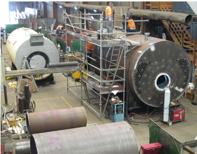
4 & 8 MW boilers under construction
